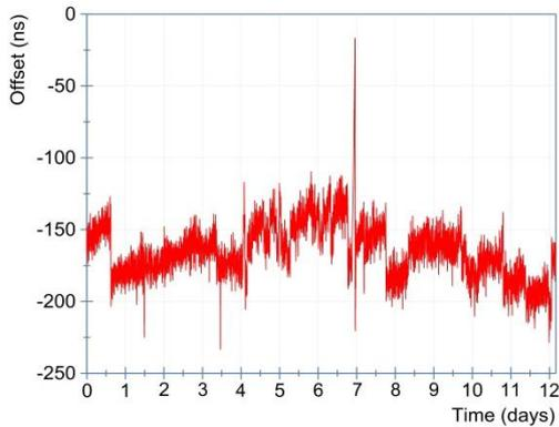
**Figure 2: Time offset between 1PPS signals from the UTC(NPL)-disciplined caesium clock and the NPLTime® client, measured over 12 days.**
