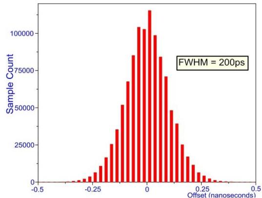
**Figure 4: Pulse to pulse (1 second) jitter characteristics of the NPLTime® signal, measured over 12 days.**
