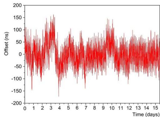
**Figure 5: Time difference between the 1PPS signals from the PTP client and the ICE GPS receiver, measured over 15 days. The mean offset has been removed.**
