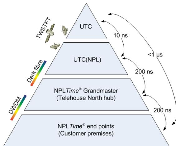
**Figure 6: Traceability pyramid relating UTC to the NPLTime<sup>®</sup> end points, with the link accuracies indicated on the right. The link from UTC(NPL), the real-time implementation of UTC, to the customer demarcation point is entirely over optical fibre and does not include GPS.**
